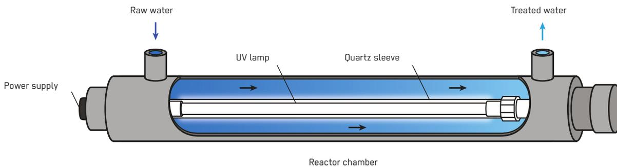
Under correct design and operational conditions, Ultraviolet (UV) Light can have anti-bacterial and anti-viral properties and can destroy pathogenic organisms in non-turbid water.
