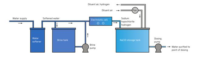
Onsite Electro-Chlorination (electrolytic generation of sodium hypochlorite) produces chlorine for disinfection through the electrolysis of aqueous sodium chloride (common salt, or NaCl). It can be produced in batch mode, converting a salt solution into sodium hypochlorite with a concentration of 6–12 g/L either in one buffer tank or in a flow-through system that continuously produces hypochlorite.
