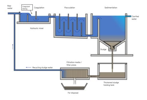
Sedimentation is a pre-treatment step used to remove suspended solids from water with varying levels of turbidity (or 'muddiness') and may involve the addition of chemicals to accelerate the process. It can be used prior to a final treatment step, such as Microfiltration (T.3), Chlorination (T.6) or Nanofiltration/Reverse Osmosis (T.15). Sedimentation can be used in all phases of an emergency.
