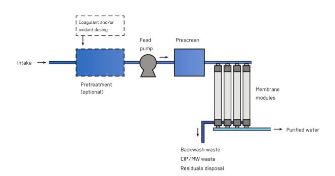
Microfiltration (MF) membranes provide excellent filtration with low final water turbidity (typically less than 0.1 NTU) and high removal levels for pathogenic protozoan cysts/ oocysts, Giardia and Cryptosporidium and bacteria. As a final treatment step, Chlorination (T.6) or Ultrafiltration (T.10) as well as Nanofiltration/Reverse Osmosis (T.15) can be used. MF is applicable in all emergency phases and at different scales (see H.4 for household scale).
