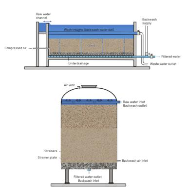
Rapid Sand Filters use coarse sand as a filtration medium to remove fine suspended solids from water with varying levels of turbidity (or 'muddiness'). It is a pre-treatment step prior to a final disinfection process, such as Chlorination (T.6), and can be used in all phases of an emergency.
