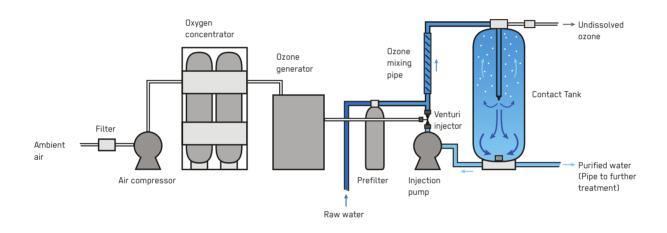
Ozonation is a water treatment process that destroys microorganisms and degrades organic pollutants through the infusion of ozone, a gas produced by subjecting oxygen molecules to a high electrical voltage. During emergencies, the technology is mainly applicable in the stabilisation and recovery phases in urban contexts, where the experience in using such systems already exists.
