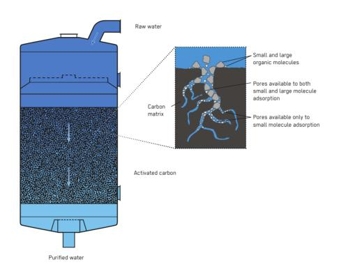
Granular Activated Carbon (GAC) is the most used adsorption method in drinking water to remove taste, odour and colour-causing compounds, natural organic matter, disinfection by-products and synthetic organic chemicals present in the source water. GAC is also used for vapour treatment to remove noxious odours and contaminants. In small-scale treatment plants, it is often used for chlorine and chloramine removal. GAC can be used in all phases of an emergency.
