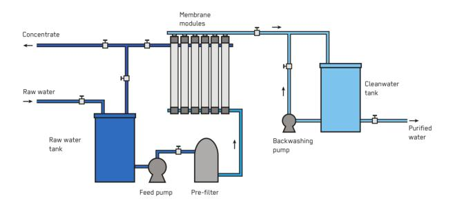
Ultrafiltration (UF) is part of the family of pressurised membrane filtration systems that can purify water from undissolved and most dissolved substances. UF is used as a final treatment step and can be applied in the acute response as well as in the stabilisation and recovery phases of emergencies.
