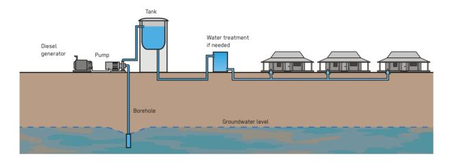
Diesel-Powered Energy Systems use diesel engines directly on site to generate the energy needed to power water pumping, transport or treatment. This energy source is more suited to acute emergencies when grid power might not be immediately available, but it is less suitable in the long term due to the mounting environmental and financial costs.
