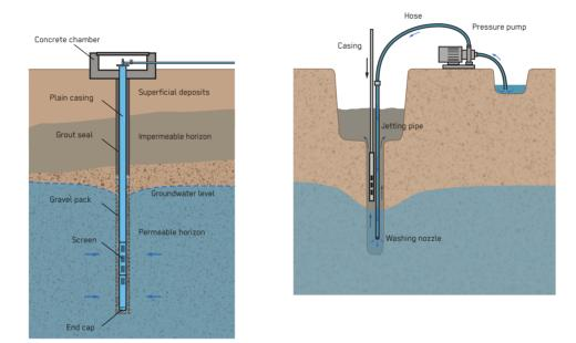
A Protected Borehole is a small diameter drilled hole that is lined and covered, with water withdrawn using a pump. Existing boreholes can be equipped quickly to provide water in the acute response phase, but new boreholes, with the exception of jetted wells, are normally reserved for the stabilisation phase, as they can take several months to organise and complete.
