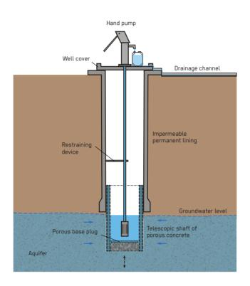
A Protected Dug Well is a large-diameter structure dug by hand that is lined and covered and allows for water abstraction using a pump. New wells are not normally considered in the acute response phase, but any existing wells can be rehabilitated quickly to provide water.
