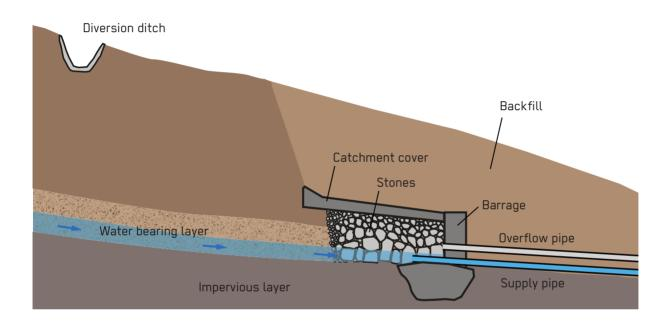
A Protected Spring Intake is designed to collect, store and transport spring water while preventing source contamination. If springs are available, the technology is suitable for all response phases.
