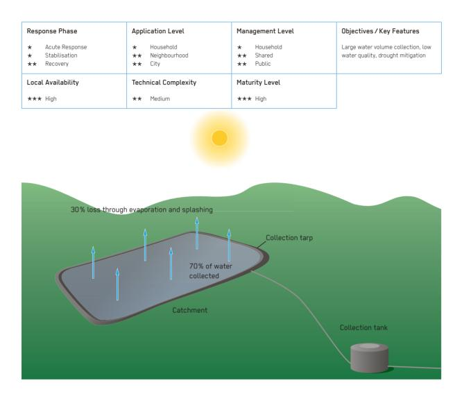
A Rainwater Ground Surface Collection system uses the ground to channel runoff water to a storage area. Although rarely done in practice during the acute response phase, any natural or artificial ground surfaces that already exist (and certain types of rapidly installed artificial surfaces such as plastic sheeting) could be useful during the rainy season. Overall, this type of rainwater catchment tends to be more suited to long-term drought mitigation or groundwater recharge.
