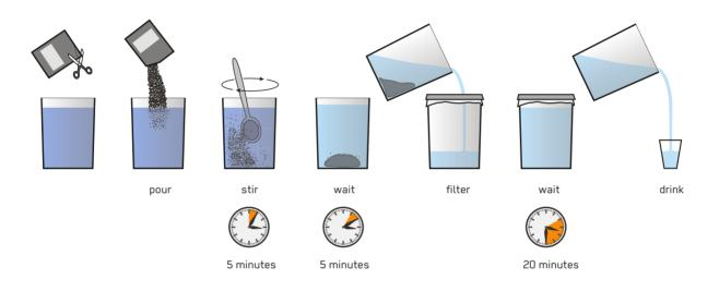
Combined Coagulation, Sedimentation and Chlorination is available for household use as small sachets of coagulant and a time-release form of chlorine. The coagulant reduces turbidity ('muddiness'), while the chlorine, which activates after some time, disinfects by inactivating pathogenic microorganisms. A single sachet treats a volume of water defined by manufacturer (e.g. 10 or 20 L) within 30 minutes.
