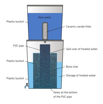
Fluoride is a groundwater contaminant naturally present in rocks and soils (commonly volcanic-derived sediments). At levels over 1.5 mg/L, it can detrimentally impact human health. As the health impacts result from prolonged consumption, Fluoride Removal is mostly relevant for the recovery phase and protracted emergencies.
