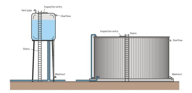
Water Storage Tanks hold large volumes of water, usually balancing supply and demand of drinking water before distribution. They are suited to all phases of an emergency.
