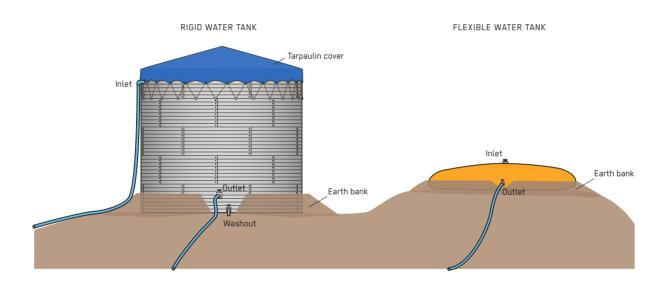
A Water Storage Tank holds large volumes of water, usually balancing supply and demand of drinking water before distribution. Transportable Water Storage Tanks (flexible or demountable rigid) can be assembled rapidly when needed. They are mainly used at the onset of an emergency to enable immediate water distribution and may also form a part of the water distribution system in the medium term.
