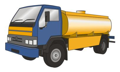
Water Trucking (or water tankering) refers to the bulk transport of water from the source to a storage facility near a distribution point. During the acute and stabilisation phases of an emergency, these trucks may be used to provide short-term transport of water to communal water points.
