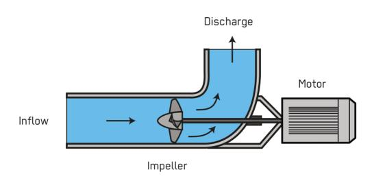
An Axial Flow Pump is a large diesel or electric motordriven pump capable of moving large volumes of water at relatively low heads. The most common uses for Axial Flow Pumps are for clearing water from flooded areas, lifting large amounts of flow within a treatment plant or water system, or for agricultural purposes, but they tend not to be used in the acute phase of an emergency.
