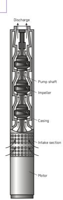
A Radial Flow Pump (also known as a centrifugal pump) is a velocity pump where a rotating impeller displaces varying amounts of water per rotation depending on the speed of rotation, which throws water outwards at right angles to the shaft. The pump is useful for all phases of an emergency.
