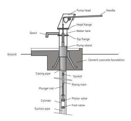
A Deep Well Piston Pump is a positive displacement pump that displaces a fixed amount of water per cycle. Water is lifted from depths of up to 90 metres with the aid of additional levers or gears. The pump is rarely suitable in the acute phase of an emergency and is instead better for long-term water supply in rural areas with low population densities.
